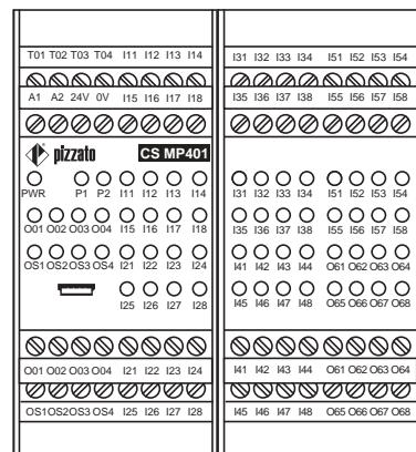
**Internal wiring diagram**
