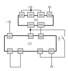
Connections with CS MF ...., CS MP .... safety modules
