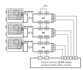
Possibility of series connection of multiple switches for simplifying the wiring of the safety system, whereby only the outputs of the last switch are evaluated by a Pizzato Elettrica safety module of the CS MP series. Both the safety-relevant evaluation and the evaluation of the signalling outputs are performed by the CS MP series.
