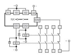
The NX •5•••1••• version, in addition to maintaining the operating and safety characteristics of the NX series, allows control of **forcibly guided NC contacts of contactors or relays** controlled by the safety outputs of the switch itself. As an alternative to the relays or contactors you can use Pizzato Elettrica expansion modules CS ME-03 (see page 267). This check is carried out via the EDM input (External Device Monitoring as defined in EN 61496-1) of the switch.
