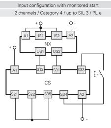
Connections with CS AR-05•••• / CS AR-06•••• safety modules Input configuration with manual start (CS AR-05••••) or monitored start (CS AR-06••••) 2 channels / Category 4 / up to SIL 3 / PL e
