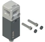
The switch is fixed directly to the metal head with two M5 screws with a hole spacing of 20 mm. The arrangement of the fixing points near the actuator's point of traction allows the loads to be distributed on a robust and compact metal structure. This ensures that the switch can withstand considerable mechanical loads without being damaged or deformed in spite of its compact dimensions. Furthermore, this type of of fixing prevents mechanical
