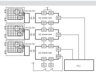
This version, with the IS safety inputs, **can be used at the end of a series** of NX switches, **up to a maximum number of 32 devices**, while maintaining the maximum PL e safety level and acc. to EN ISO 13849-1 and SIL 3 safety level acc. to EN IEC 62061.
