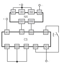
Connections with CS AT-0 ····· / CS AT-1 ···· safety modules
